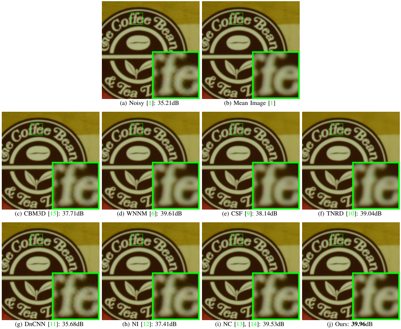
Fig. 3: Denoised images of a region cropped from the real-world noisy image “Nikon D800 ISO 1600 B2” [1] by different methods. The images are better viewed by zooming in on screen.
