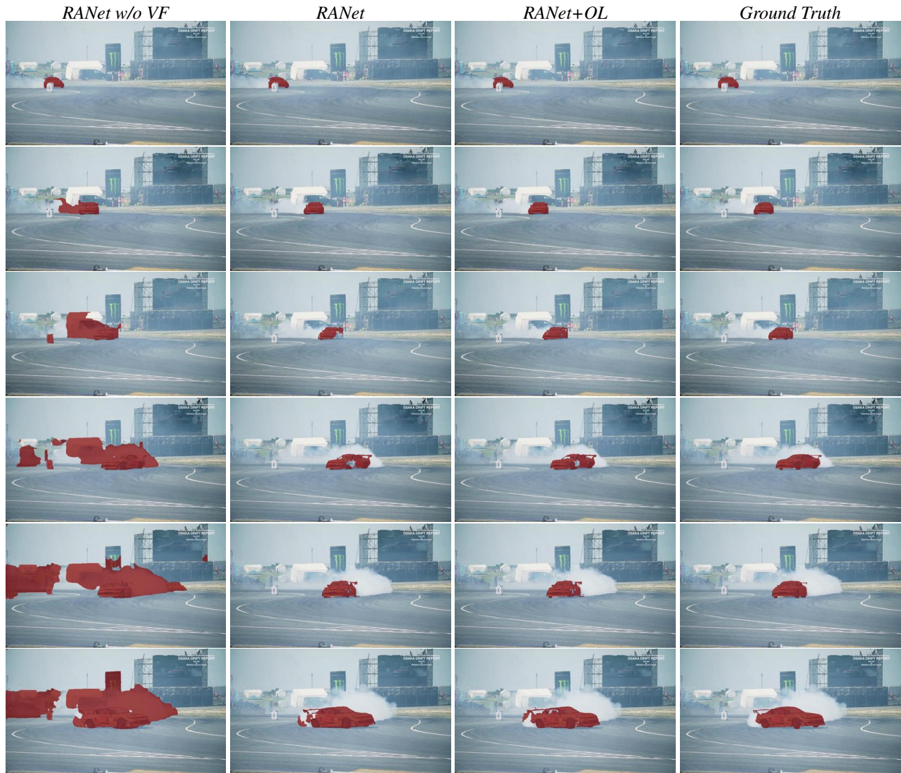
Figure 4: Comparison results of RANet with different training strategies, on sequence drift-chicane from DAVIS 16 dataset [4]. From left to right, the results are from RANet trained only on static images ( RANet w/o VF ), RANet trained on static images and fine-tuned on videos ( RANet ), RANet boosted by online learning ( RANet+OL ), and Ground Truth .
